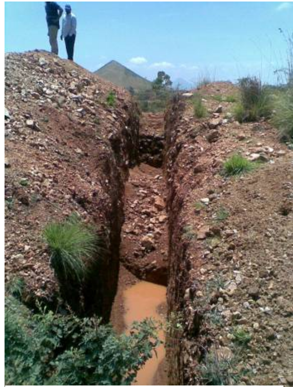
Photo 3 - Geomysore trench cut across NE trending silicified zone in brecciated felsic schist.
